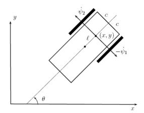
The angle of rotation about the vertical is denoted by  $\theta$ , and the positions of the wheels are characterized by angles  $\psi_1$  and  $\psi_2$ . We shall generally assume that the intersection point (x,y) of the horizontal symmetry axis of the carriage with the line which connects the two wheels is not necessarily the centre of mass of the system, but lies at a distance  $\ell$  from it.
