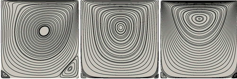
Figure 1: Streamlines for Re = 400 and (left to right) \alpha = 0 , \alpha = 0.01 and \alpha = 5 .
