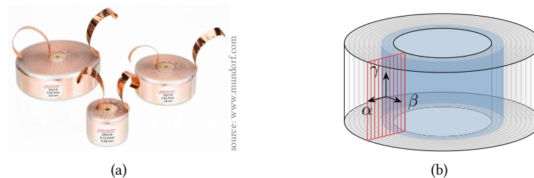
Figure 1: (a) shows three foil windings, and (b) shows the representation of a foil winding with a local coordinate system on a cross section (red) and with cut \Gamma(\alpha) (blue).
